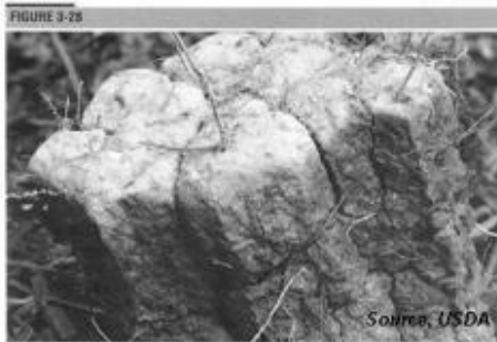
A cluster of strong medium columnar peds. The cluster is about 133 mm across.
